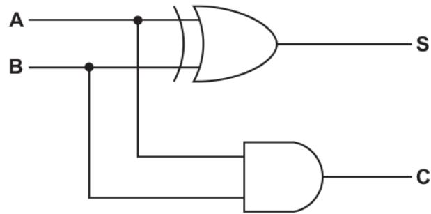
The logic circuit above has two inputs (A, B) and two outputs (S, C).
